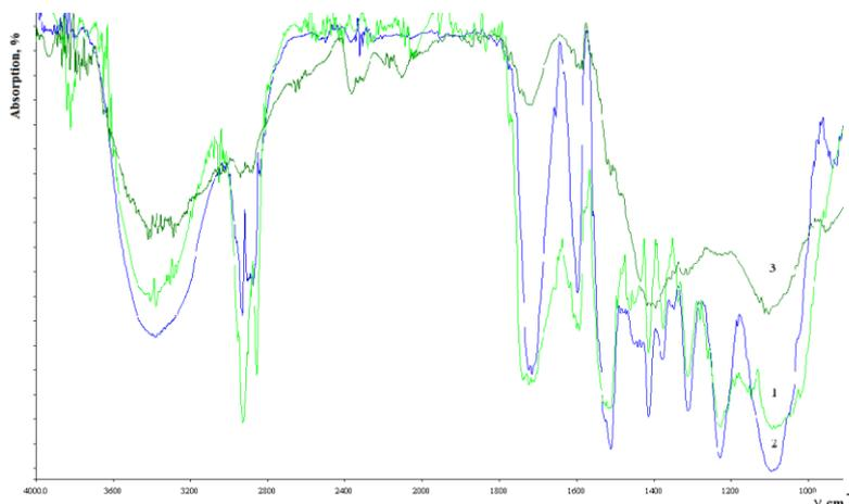
**Figure 3: IR spectra of the reference PU foam (1), PU foam after 606-hour UV radiation (2), PU foam sample after the oxidation reaction at  $230\text{ }^{\circ}\text{C}$  (3)**
