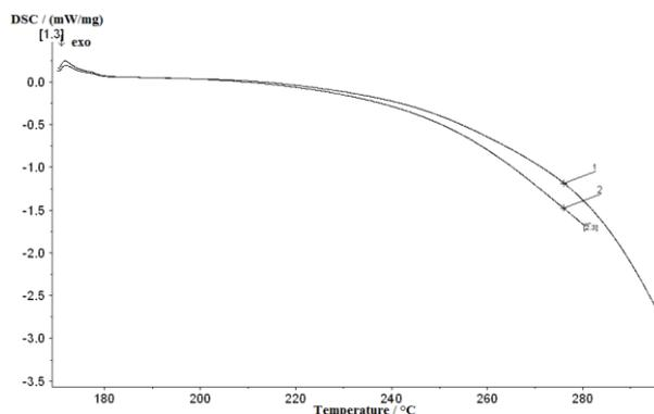
**Figure 2: OOT for the samples of reference PU foam (1) and PU foam after 550-hour UV exposure (2)**
