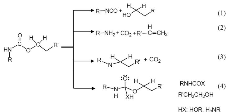
**Figure 4: Degradation mechanism of urethane segment**
