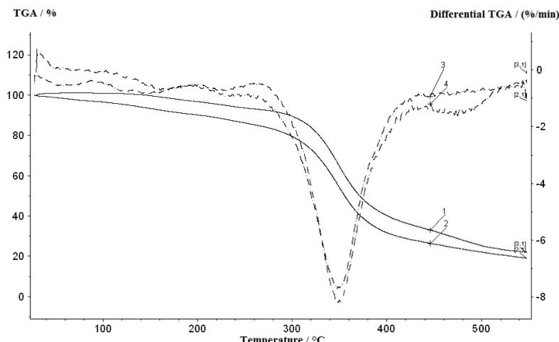
**Figure 1: Thermogravimetric analysis of the reference PU foam (TGA curve - 1, differential TGA curve - 3) and PU foam samples after 606-hour UV exposure (TGA curve - 2, differential TGA curve - 4)**
